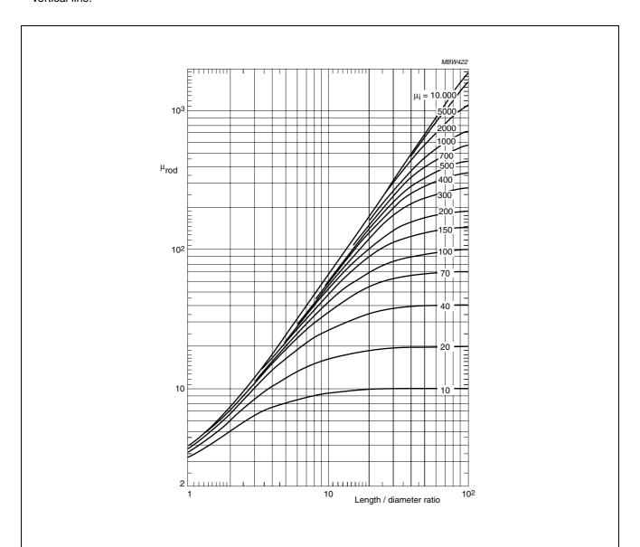
Fig.64 Rod permeability ( $\mu_{rod}$ ) as a function of length to diameter ratio with material permeability as a parameter.
