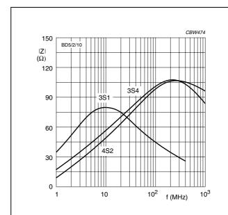
Fig.47 Impedance as a function of frequency for material grades 3S1, 3S4 and 4S2; bead size  $5 \times 2 \times 10$  mm.
