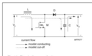
Fig.13 Circuit diagram of a boost or up converter
