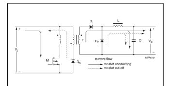
Fig.15 Circuit diagram of a forward converter.
