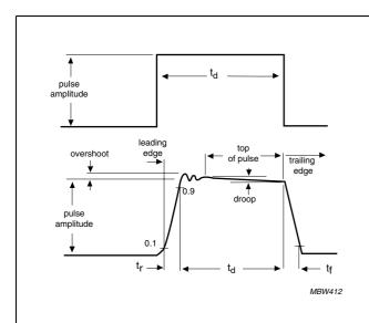
Fig.10 An ideal rectangular pulse and the main pulse distortions that may be introduced by a transformer.
