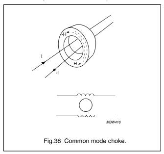
To avoid the conduction of switching noise from a SMPS into the mains, an input filter is generally necessary. The magnetic circuit in these filters is usually a pair of U cores or a ring core.
