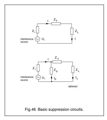
Suppressors are used in series with the load impedance. They provide a low impedance for the wanted signal, but a high impedance for the interfering, unwanted, signal.
