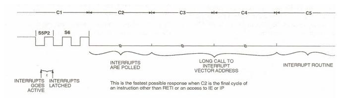
Thus the processor acknowledges an interrupt request by executing a hardware generated LCALL to the appropriate servicing routine.
