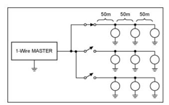
The example above appears like a star topology network with a radius of 150m and a weight of 450m. However, when each switched path is considered individually, the network is actually a linear topology and the weight is only 150m.
