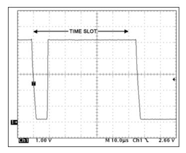
This image shows a Read One or Write One time slot. The master pulls the bus low for about  $10\mu$ s and then releases it. Note the slew-rate-controlled fall time. The time slot lasts for about  $70\mu$ s, after which another time slot occurs. Note that the time base is changed to  $10\mu$ s per division.
