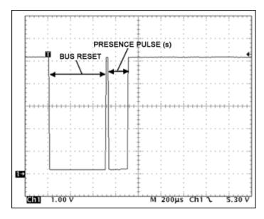
This image also shows a bus reset/presence-detect sequence. The master pulls the bus low for 480µs; all the devices on the bus recognize this as a reset operation. Slaves respond to a bus reset by issuing a presence pulse. Multiple slaves generate their presence pulses during the same period, and the pulses overlap to form a single pulse. (Note that the time base is 200µs per division.)
