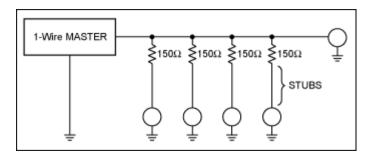
The most successful implementation of this concept uses  $150\Omega$  resistors at each point where a stub is connected to the main trunk. This value reduces the mismatch at the connection point by about 20%, and attenuates the resulting stub reflections by about 40%. However, the added resistance also degrades noise immunity by about 80%, so caution must be observed. Tests have also shown good performance using  $100\Omega$  resistor values, which do not degrade noise immunity quite as much.
