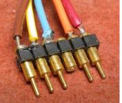
On the programmer side, the developer must use the connector provided by the programmer. If no ICSP connector is provided, the builder can use a machine pin DIP socket as a plug to connect to the programmer's PIC socket. The less expensive tin solder tail sockets will not connect cleanly into the PIC socket and are not as durable.
