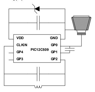
Figure 8. The iGlassware glass schematic.
