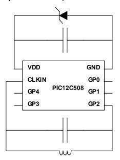
Figure 6. Ignatov's PIC-based RFID tag [6].
