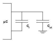
Figure 4. The microcontroller-based capacitance measurement circuit.
