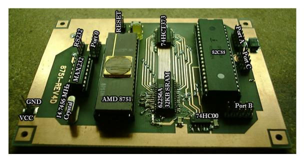
Since taking this picture, I've switched out the processor and crystal in favor of a 22MHz, flash based set. Here's the design of the board:
