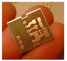
A simple drill press and wire gauge bits seem to work well. Be sure to change the speed of the drill press, as the usually come from the store in the lowest speed. I use the maximum speed of my press, around 3200 rpm. The slower speeds are good for wood, but when cutting metals it does more tearing and less cutting.
