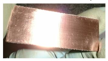
tend to go in one direction, and then switch 90° every now and then. The idea is to remove all oxidation on the surface of the circuit board and provide a regular surface structure for the adhesion of the toner when it's melted. Get rid of as much discoloration on the board as is possible.
