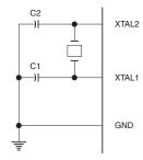
Note: C1, C2 =  $30 \text{ pF} \pm 10 \text{ pF}$  for Crystals =  $40 \text{ pF} \pm 10 \text{ pF}$  for Ceramic Resonators
