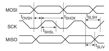
**Table 21-1.** Serial Programming Characteristics,  $T_A = -40$ · C to 85· C,  $V_{CC} = 4.0$  - 5.5V (Unless Otherwise Noted)
