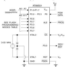
Figure 17-1. Programming the Flash Memory (Parallel Mode)
