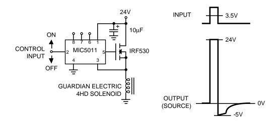
Figure 4. Clamping Inductive Transients
