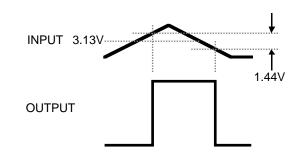
Figure 5. Adding Hysteresis to Suppress Oscillations with Slow-Moving Inputs
