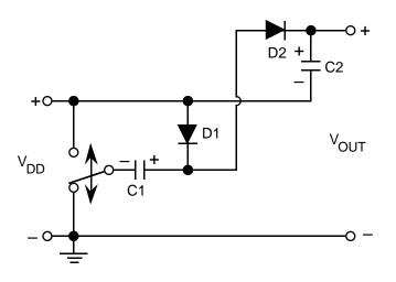
Figure 1. Charge Pump Voltage Doubler
