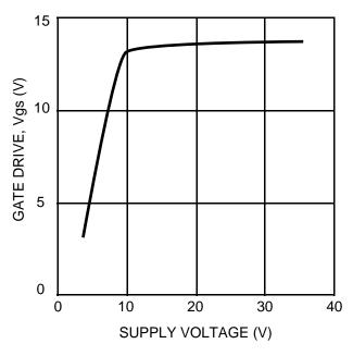
Figure 3. Gate Drive vs. Supply Voltage
