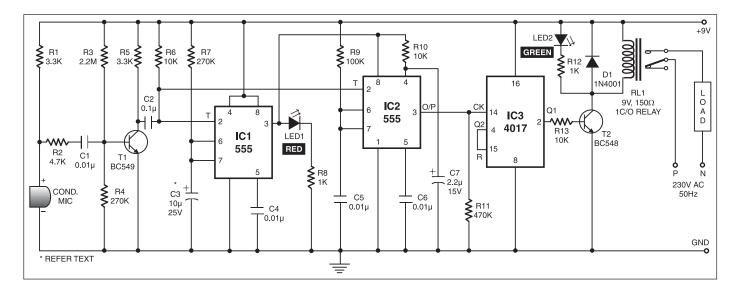
to pin 2 of IC1 and IC2, triggering both the ICs. IC1, commonly used as a timer, is wired here as a monostable multivibrator. Trigging of IC1 causes pin 3 to go high and it remains high for a certain time period
