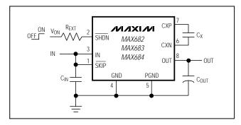
Figure 5. Standard Operating Circuit
