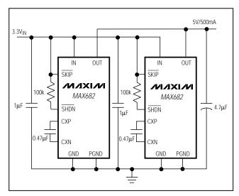
Figure 6. Paralleling Two MAX682s
