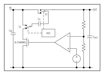
Figure 4. Constant-Frequency-Mode Regulation
