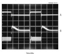
A: LOAD CURRENT:  $I_{LOAD} = 5$ mA TO 250mA, 500mA/div B: OUTPUT VOLTAGE:  $\overline{SKIP} = HIGH$ ,  $I_{\overline{SHDN}} = 22\mu$ A, 100mV/div, MAX682
