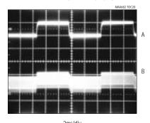
A: INPUT VOLTAGE:  $V_{IN}=3.1V$  TO 3.6V, 500mV/div B: OUTPUT VOLTAGE:  $\overline{SKIP}=HIGH$ ,  $I_{SHDN}=22\mu A$ ,  $I_{LOAD}=250mA$ , 50mV/div, MAX682
