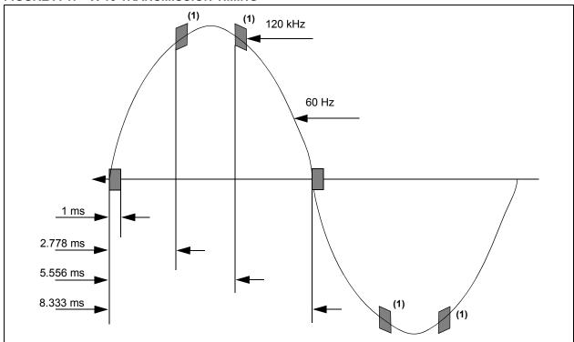
**Note 1:** These 120 kHz carrier bursts are timed to coincide with the zero-crossing of the other phases, when implemented.
