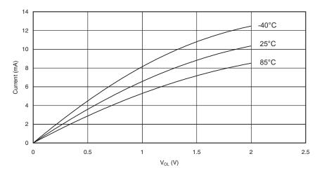
Figure 154. Reset Pin as I/O – Pin Sink Current vs. Output Voltage ( $V_{CC}$  = 2.7V)
