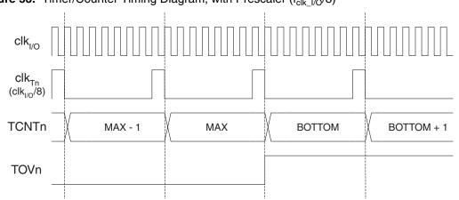
**Figure 53.** Timer/Counter Timing Diagram, with Prescaler ( $f_{clk_l/O}/8$ )
