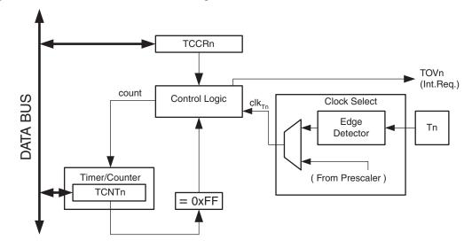
RegistersThe Timer/Counter (TCNT0) is an 8-bit register. Interrupt request (abbreviated to Int. Req. in the<br/>figure) signals are all visible in the Timer Interrupt Flag Register (TIFR). All interrupts are individ-<br/>ually masked with the Timer Interrupt Mask Register (TIMSK). TIFR and TIMSK are not shown in<br/>the figure since these registers are shared by other timer units.
