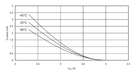
**Figure 151.** Reset Pin as I/O – Pin Source Current vs. Output Voltage ( $V_{CC} = 5V$ )
