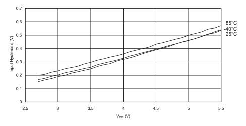
Figure 158. Reset Pin as I/O – Input Threshold Voltage vs.  $V_{CC}$  (V<sub>IH</sub>, I/O Pin Read as "1")
