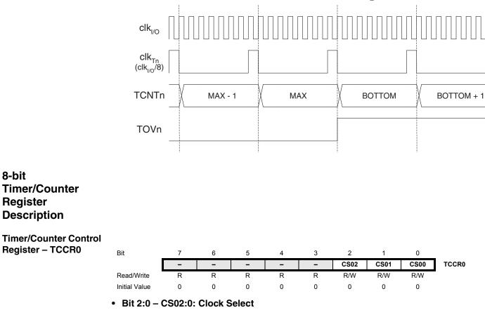
Figure 29. Timer/Counter Timing Diagram, with Prescaler ( $f_{clk\_l/O}/8$ )
