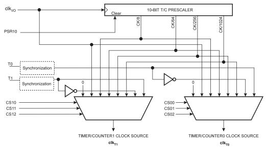
Figure 31. Prescaler for Timer/Counter0 and Timer/Counter1<sup>(1)</sup>
