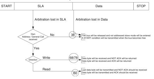
Figure 88. Possible Status Codes Caused by Arbitration
