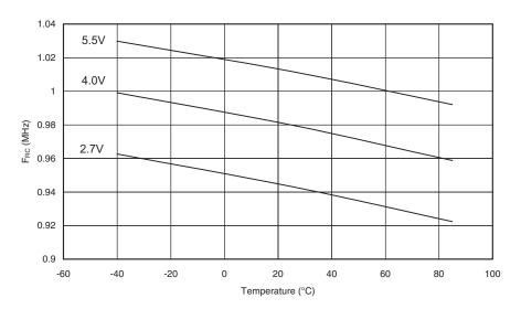
Figure 180. Calibrated 1MHz RC Oscillator Frequency vs.  $\rm V_{\rm CC}$
