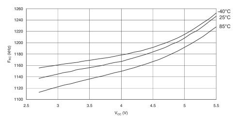
Figure 170. Calibrated 8MHz RC Oscillator Frequency vs. Temperature
