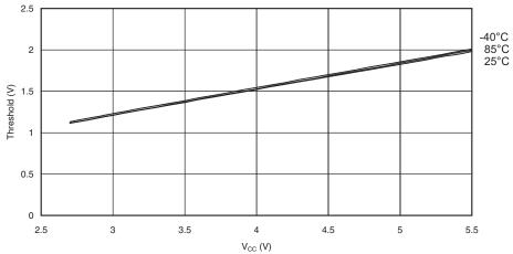
Figure 156. I/O Pin Input Threshold Voltage vs.  $V_{CC}$  (V<sub>IL</sub>, I/O Pin Read as "0")
