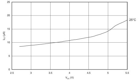
Figure 186. Watchdog Timer Current vs.  $V_{CC}$
