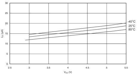
Figure 183. ADC Current vs.  $V_{CC}$  (AREF = AV<sub>CC</sub>)
