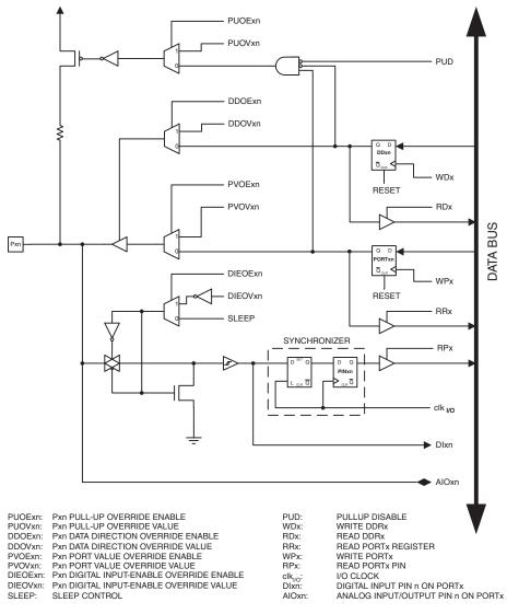
Figure 25. Alternate Port Functions<sup>(1)</sup>
