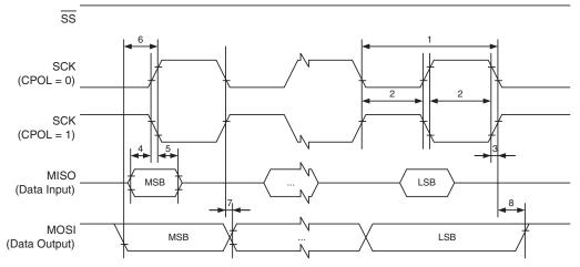
Figure 117. SPI interface timing requirements (Slave Mode)
