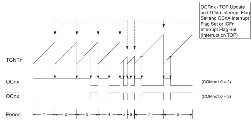
The Timer/Counter Overflow Flag (TOV1) is set each time the counter reaches TOP. In addition the OCF1A or ICF1 Flag is set at the same timer clock cycle as TOV1 is set when either OCR1A or ICR1 is used for defining the TOP value. If one of the interrupts are enabled, the interrupt handler routine can be used for updating the TOP and compare values.
