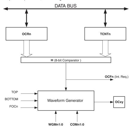
Figure 47. Output Compare Unit, Block Diagram
