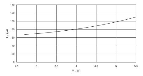
Figure 140. Standby Supply Current vs. V<sub>CC</sub> (4MHz Xtal, Watchdog Timer Disabled)
