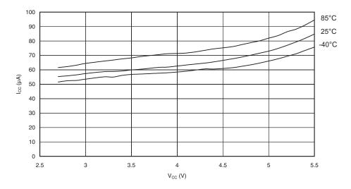
Figure 188. Programming Current vs.  $V_{CC}$
