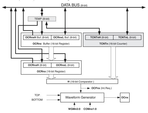
Figure 35. Output Compare Unit, Block Diagram
