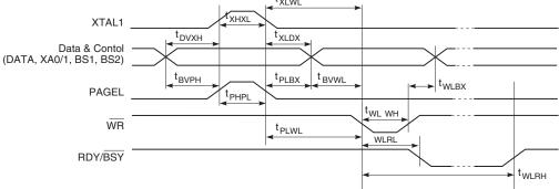
Figure 110. Parallel Programming Timing, Loading Sequence with Timing Requirements<sup>(1)</sup>
