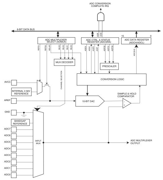
The ADC converts an analog input voltage to a 10-bit digital value through successive approximation. The minimum value represents GND and the maximum value represents the voltage on the AREF pin minus 1 LSB. Optionally,  $AV_{CC}$  or an internal 2.56V reference voltage may be connected to the AREF pin by writing to the REFSn bits in the ADMUX Register. The internal voltage reference may thus be decoupled by an external capacitor at the AREF pin to improve noise immunity.
