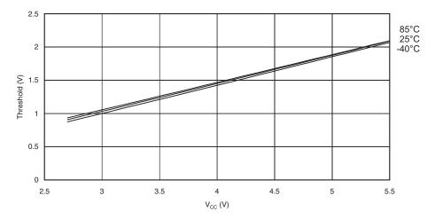
Figure 160. Reset Pin as I/O – Pin Hysteresis vs.  $V_{\text{CC}}$
