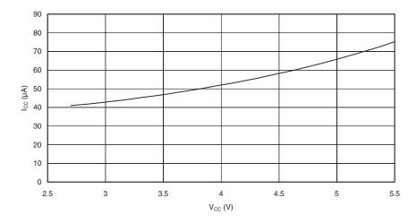
Figure 138. Standby Supply Current vs. V<sub>CC</sub> (2MHz Xtal, Watchdog Timer Disabled)
