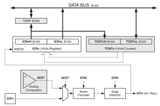
Figure 34. Input Capture Unit Block Diagram
