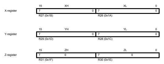
Figure 4. The X-register, Y-register and Z-Register
