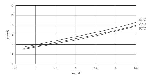
Figure 122. Active Supply Current vs. V<sub>CC</sub> (Internal RC Oscillator, 2MHz)
