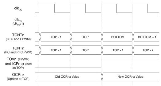
Figure 43. Timer/Counter Timing Diagram, no Prescaling
