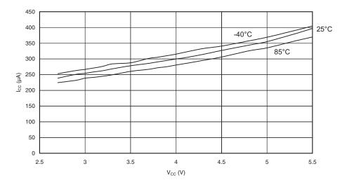
Figure 184. AREF External Reference Current vs.  $V_{CC}$
