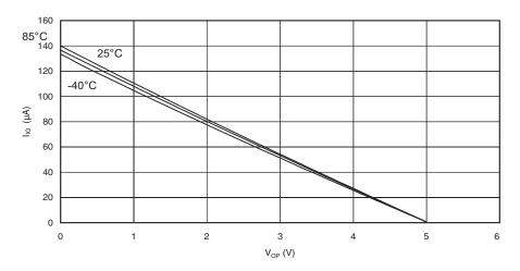
Figure 144. I/O Pin Pull-up Resistor Current vs. Input Voltage ( $V_{CC} = 2.7V$ )
