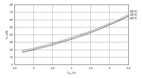
Power-save SupplyFigure 134.Power-save Supply Current vs. V<sub>CC</sub> (Watchdog Timer Disabled)Current
