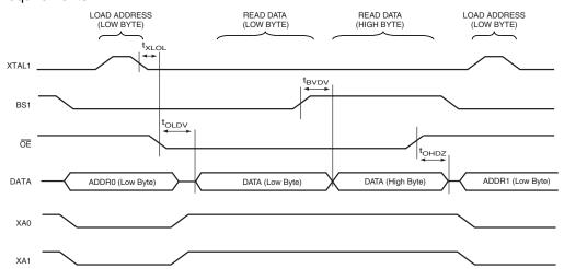
**Figure 111.** Parallel Programming Timing, Reading Sequence (within the same Page) with Timing Requirements<sup>(1)</sup>
