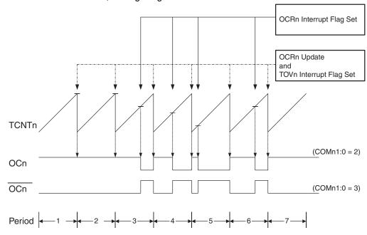
Figure 50. Fast PWM Mode, Timing Diagram
