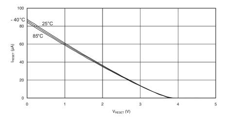
Figure 146. Reset Pull-up Resistor Current vs. Reset Pin Voltage ( $V_{CC} = 2.7V$ )
