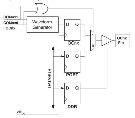
Figure 36. Compare Match Output Unit, Schematic
