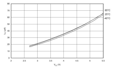
Figure 187. Analog Comparator Current vs.  $V_{CC}$
