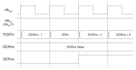
Figure 42 shows the same timing data, but with the prescaler enabled.
