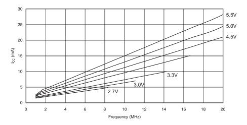
Figure 120. Active Supply Current vs. V<sub>CC</sub> (Internal RC Oscillator, 8MHz)
