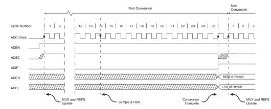
Figure 92. ADC Timing Diagram, First Conversion (Single Conversion Mode)
