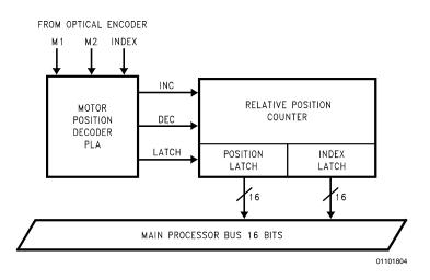
FIGURE 4. LM628/629 Motor Position Decoder
