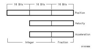
FIGURE 6. Position, Velocity and Acceleration Registers
