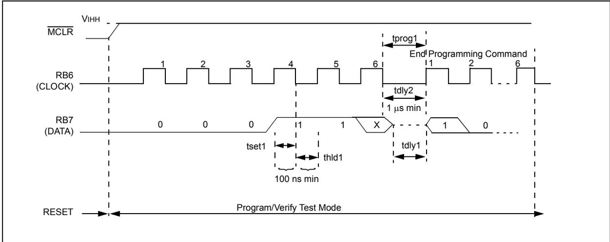
**FIGURE 6-8: BULK ERASE PROGRAM MEMORY COMMAND (PROGRAM/VERIFY)**
