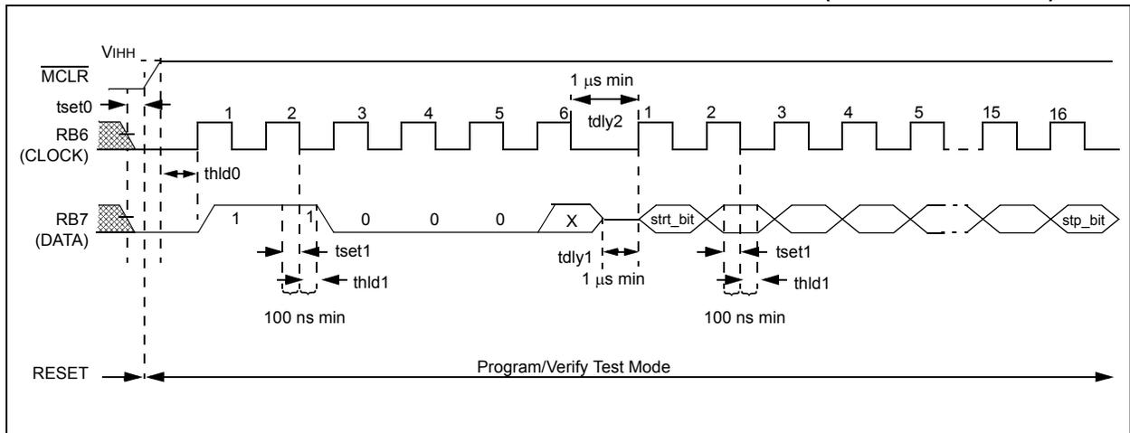
**FIGURE 6-3: READ DATA FROM PROGRAM MEMORY COMMAND (PROGRAM/VERIFY)**
