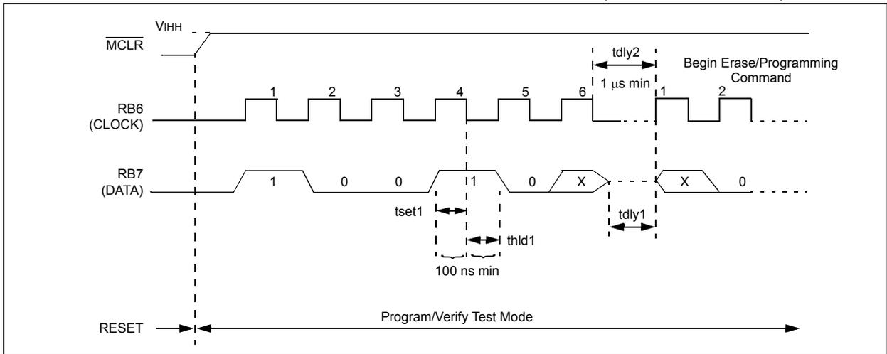
**FIGURE 6-9: BULK ERASE DATA MEMORY COMMAND (PROGRAM/VERIFY)**
