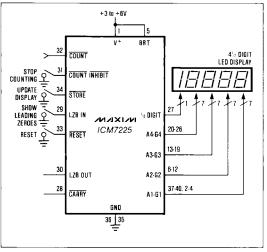
Figure 2. Simple 41/2 Digit Event or Unit Counter with LED Display
