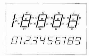
Figure 5. Segment Assignment and Display Font
