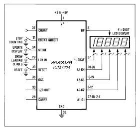
Figure 1. Simple 41/2 Digit Event or Unit Counter with LCD Display
