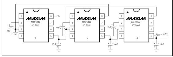
Figure 12. Cascading MAX1044/ICL7660 for Increased Output Voltage
