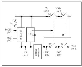
Figure 4. MAX1044 and ICL7660 Functional Diagram
