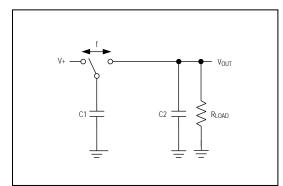
Figure 3a. Switched Capacitor Model
