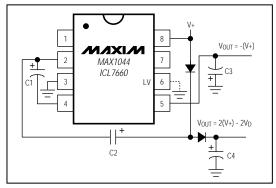
Figure 11. Combined Positive and Negative Converter
