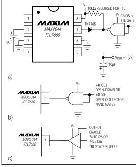
Figure 14a-14c. Shutdown Schemes for MAX1044/ICL7660
