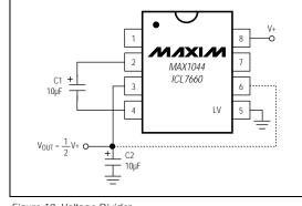
Figure 10. Voltage Divider
