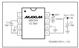
Figure 5. Basic Negative Voltage Converter
