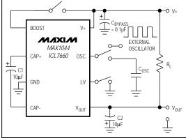
Figure 1. Maxim MAX1044/ICL7660 Test Circuit
