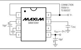
Figure 6. Negative Voltage Converter with C<sub>OSC</sub> and BOOST
