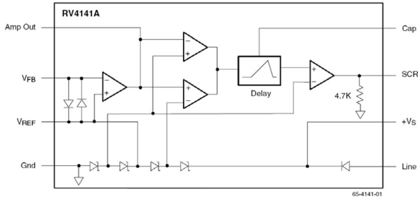
Figure 1. Block Diagram
