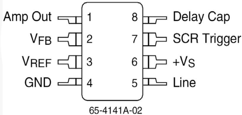
Figure 2. Pin Assignment
