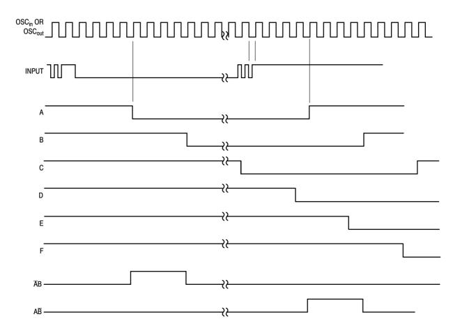
Figure 10. Multiple Output Signal Timing Diagram
