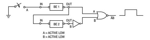
Figure 9. Single Pulse Output Circuit
