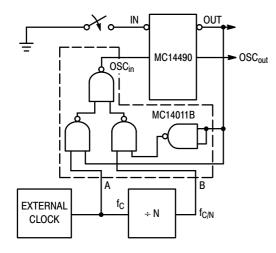
Figure 6. Fast Attack/Slow Release Circuit
