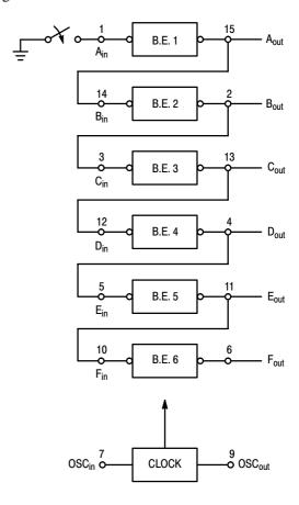
**Figure 8. Multiple Timing Circuit Connections**
