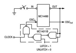
Figure 7. Latched Output Circuit
