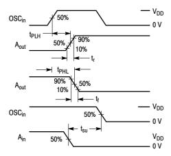
Figure 1. Switching Waveforms
