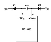
Figure 2. Discharge Protection During Power Down
