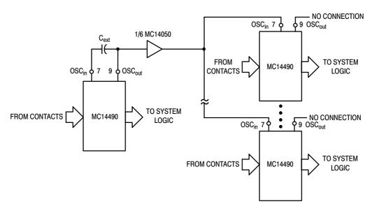
Figure 5. Typical Single Oscillator Debounce System
