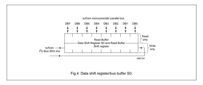
In receiver mode the data from the shift register is copied to the read buffer during the acknowledge phase. Further reception of data is inhibited (SCL held LOW) until the S0 read buffer is read (see Section 6.8.1.1).
