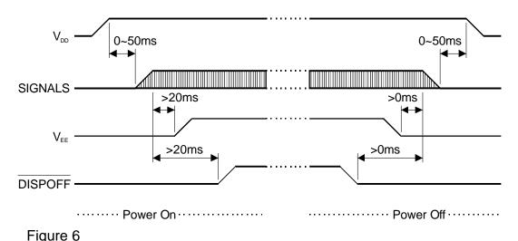
generator with a logic signal. Using this signal the generator IC is kept in the shutdown mode until  $V_{DD}$  is stable and the LCD controller has been initialized and has started to scan the display. At this time  $V_{EE}$  can be applied to the display safely. The turn off procedure is just the reverse of the turn on procedure.
