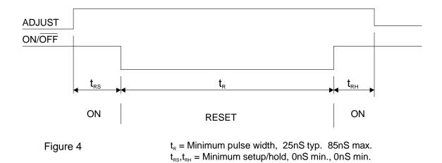
A RESET is accomplished by setting the ADJUST line high and then setting the ON/OFF line low for longer than 400nS. See Figure 4.
