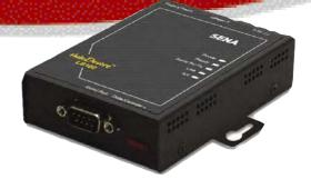
The HelloDevice Lite Series, LS100/LS100W is a costeffective Serial Device Server that makes your legacy serial devices manageable via industry-standard 10Base-T Ethernet or WiFi network. Based on open network protocols such as TCP/IP, it gives you ultimate flexibility to your serial devices. The unique hardware and software design enables you to connect RS232 serial devices to Ethernet network at a minimal transition cost.
