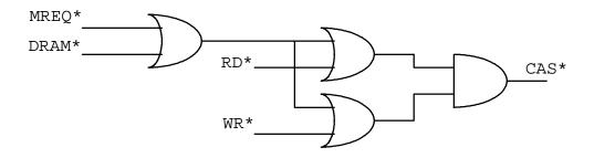
Fig 8. Circuit to generate CAS for Z80.
