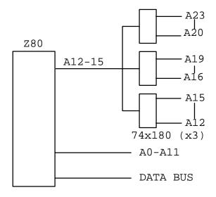
Fig 17. Z80 CPU with external MMU.
