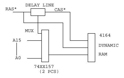
Figure 2. Basic DRAM Timing Generation
