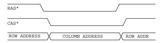
Figure 3. Timing for circuit in Fig 2.
