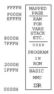
Fig 19. Possible mapping for Z80 MMU
