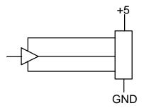
Fig 27. Correct power routing.
