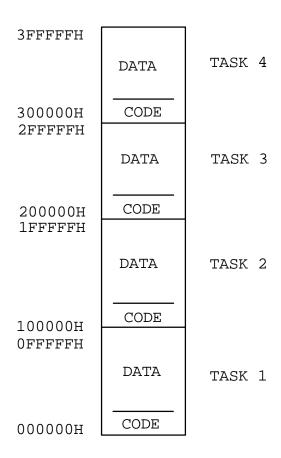
Fig 20 - Memory layout for multi-tasking
