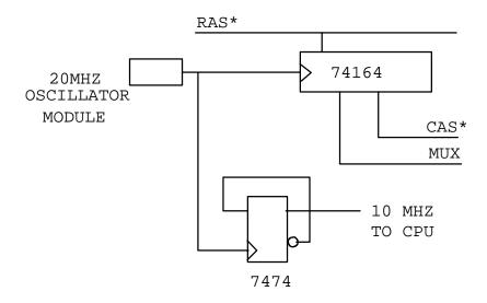
Fig 4. Shift Register Timing Generation.
