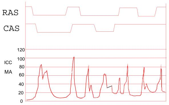
Fig 25 - Current waveform of DRAM access.
