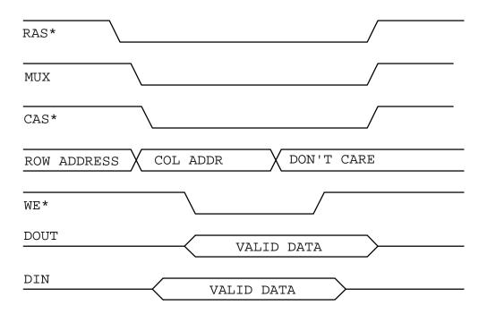
Fig 5. Basic DRAM WRITE timing.
