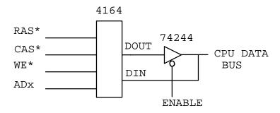
Fig 6. Separate I/O implementation.
