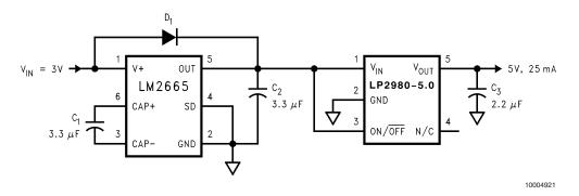
FIGURE 5. Generate a Regulated +5V from +3V Input Voltage
