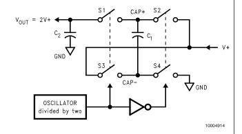
FIGURE 2. Voltage Doubling Principle
