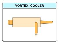
This one is nothing but a Tee shaped pipe. Blow air in the middle arm, and hot air comes out one end and cold air out the other. To -40 degrees and tons of refrigeration.
