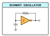
What is the simplest possible electronic oscillator you can build? For square waves, the *Schmidt Oscillator* wins hands down. It uses 2-1/6 parts, always self starts, is fairly temperature and voltage stable, and outputs more or less symmetric square waves. This dude can be micropower at low frequencies and drives fairly heavy loads.
