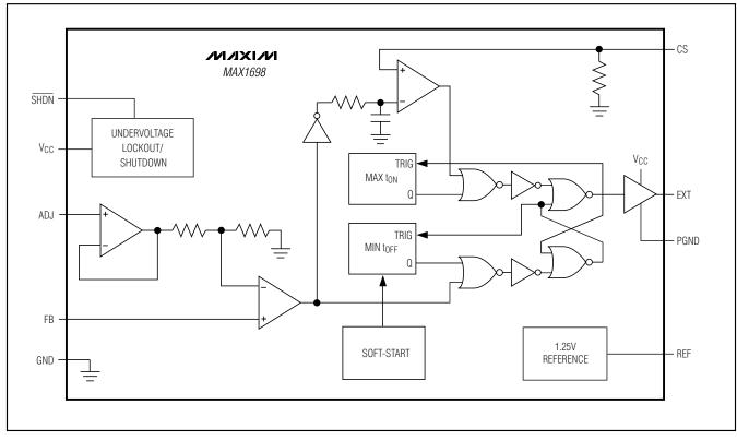
Figure 1. Functional Diagram
