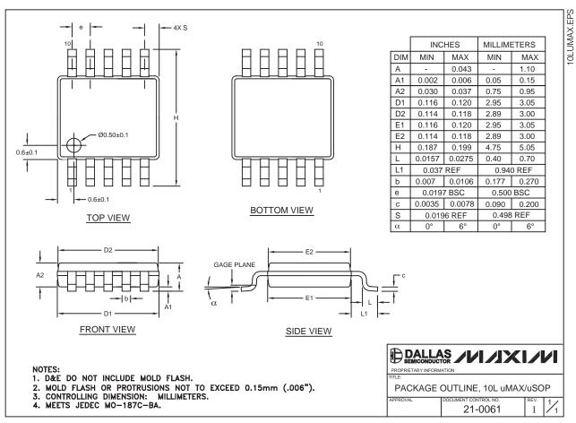
Note: The MAX1698 does not have an exposed pad.
