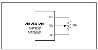
Figure 3. Adjusting LED Current
