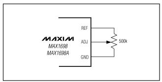
Figure 3. Adjusting LED Current
