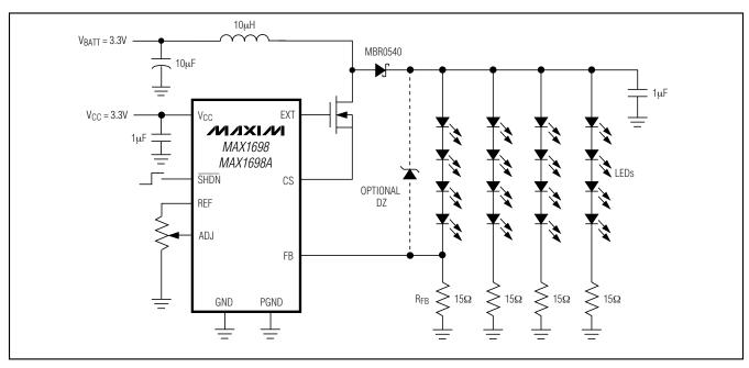
Figure 2. Typical Operating Circuit
