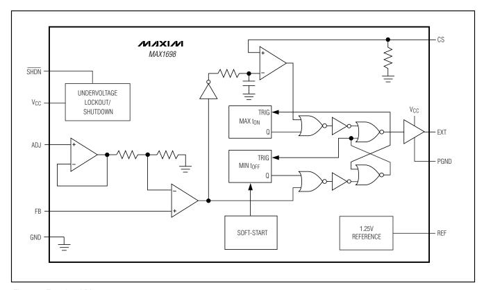
Figure 1. Functional Diagram
