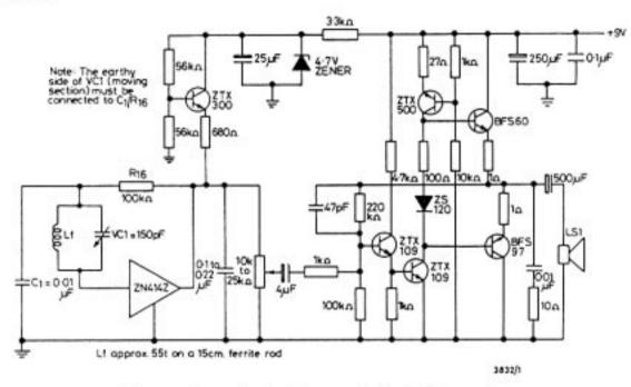
The complete circuit diagram of the Triffid receiver
