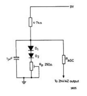
$D_1 = D_2 = Any$  general purpose silicon diode  $R_p = Optional sensitivity control, a$ recommended value being 250 $\Omega$ .
