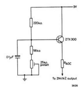
Current consumption is virtually that which is taken by the ZN414Z (0.3mA)
