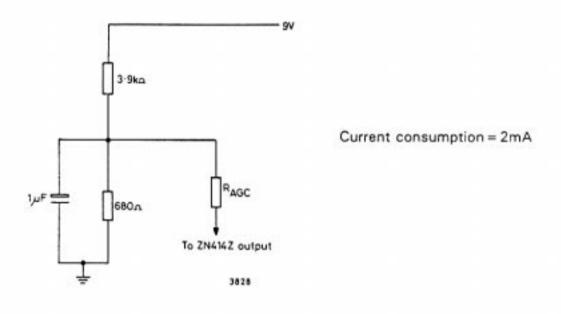
Note: Replacing the  $680\Omega$  resistor with a  $500\Omega$  resistor and a  $250\Omega$  preset, sensitivity may be adjusted and will enable optimum reception to be realised under most conditions.
