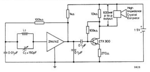
$L_1 = 80$  turns of 0.3mm dia. enamelled copper wire on a 5cm or 7.5cm long ferrite rod. Do not expect to adhere rigidly to the coil-capacitor details given. Any value of  $L_1$  and  $C_1$  which will give a high 'Q' at the desired frequency may be used.
