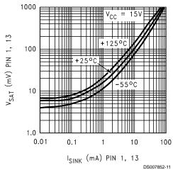
Discharge Transistor (Pin 1, 13) Voltage vs. Sink Current
