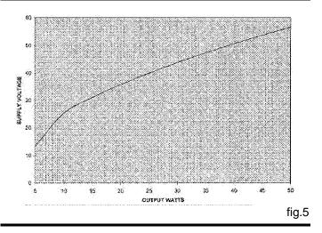
Figure 5 shows the supply voltage requirements versus output power. This voltage ranges from about plus and minus fifteen volts for a five watt output to plus and minus fifty-seven volts for a fifty watt output.
