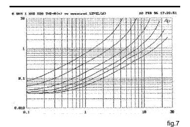
Figure 7 shows a family of distortion curves versus output power for several different supply levels, from about a 4 watt rating to 30 watt rating. These curves were taken at one kiloHertz, but I did not find significant variation versus frequency. The prototype amplifier went up to 30 watts with 45 volt supply rails, and drew about 700 watts per channel.
