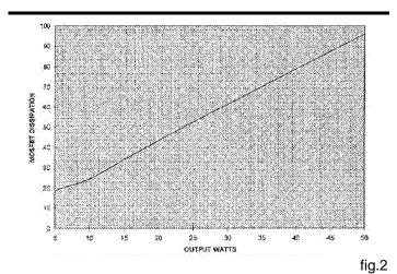
Heat sinking for these Mosfets is very important to their reliability. The rule of thumb for heat sinking is that you should be able to touch the heat sink during operation. This requirement limits the temperature to about 55 degrees Centigrade, and assures a chip temperature within the device's ratings. You can run the devices at higher temperatures, but I would suggest having some spares, as it will reduce their operating life.
