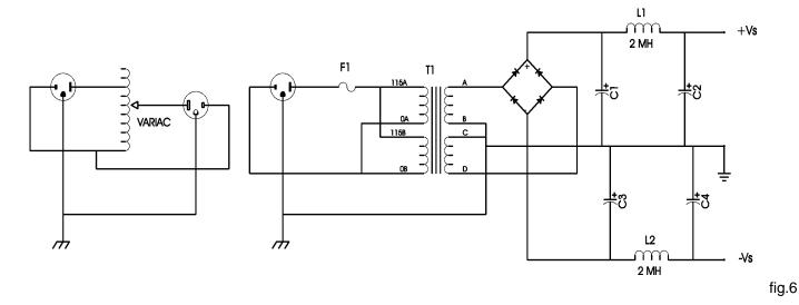
values can be achieved by paralleling capacitors if necessary. Lower impedances at high frequencies can be achieved by paralleling film capacitors with these computer-grade electrolytics.
