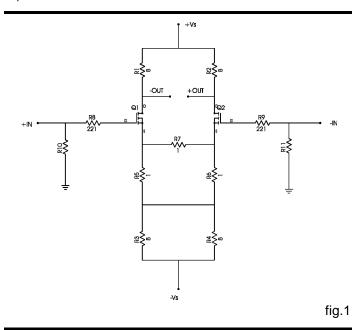
The circuit is supplied by two supply voltages +Vs and -Vs, and the loudspeaker is driven across the drain connections of the Mosfets.
