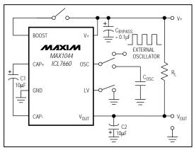
Figure 1. Maxim MAX1044/ICL7660 Test Circuit
