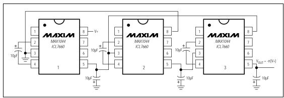
Figure 12. Cascading MAX1044/ICL7660 for Increased Output Voltage
