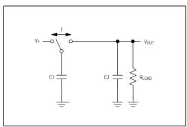
Figure 3a. Switched Capacitor Model
