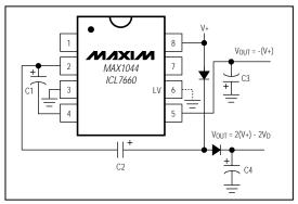
Figure 11. Combined Positive and Negative Converter
