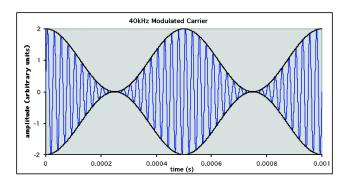
The envelope function in this case is  $E(t)=1+\cos(2^{*}\pi^{*}2kHz^{*}t)$ , or  $-[1+\cos(2^{*}\pi^{*}2kHz^{*}t)]$ . With an amplitude modulated carrier, the envelope is simply proportional to the modulation signal, plus an offset constant. Also notice that the lower envelope is a mirror image of the upper one.
