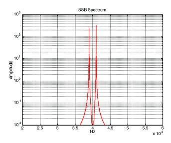
For a 2kHz audio signal, only 2kHz of ultrasonic bandwidth is required.
