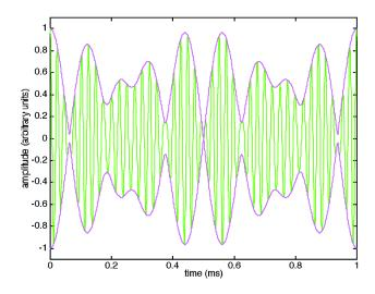
Next, the ideal envelope (square-rooted audio) for equal-amplitude 7kHz and 9kHz signals is shown on the same plot as the uncorrected SSB envelope:
