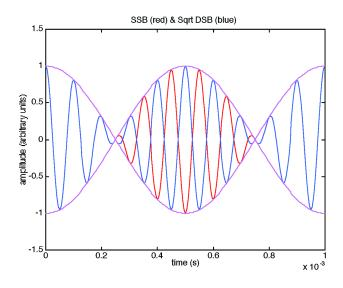
The blue DSB line lies on top of the red line when their values are the same, so when only the blue line can be seen, the red trace is underneath it. Both of these methods give the same envelope that will demodulate into a single, distortion-free audio signal (in this case, 2kHz). However, the spectrums required to generate these two envelopes are vastly different. Lets look at them. Here is the SSB spectrum with two frequencies:
