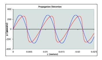
The values used for the graph above are as follows:SPL of the pure sinewave: 140dB (re. 20μ Pa)Frequency: 40.0kHzPropagation time: 0.0013 sec.
