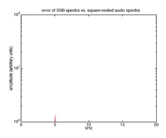
This suggests that by utilizing a recursive scheme we can correct a SSB envelope without requiring any additional bandwidth. Note, as opposed to DSB, all of the correction sidebands fall within the bandwidth of the original audio input signal. Also, as can be seen, the amount of error occurrence, as a percent, falls with each recursive correction step used.
