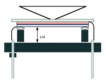
When a voltage is applied across the pins (that are protruding downward), the red element gets longer while the blue one shortens, causing a bent in the bimorph. When the polarity changes, the opposite bend occurs. The maximum displacement change is in the center of the element where the cone is attached. This way, the cone undergoes maximum displacements. Also, the outer edge of the cone moves as much as three times further than the inner portion as it flexes.
