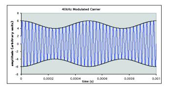
To get this signal, the carrier amplitude in the figure shown above, was simply increased by a factor of five. This results in a decreased modulation percent. The earlier case was 100% modulated, where this one is only at 20%.
