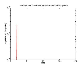
You can see that the only error term is at 2kHz. It can be proven mathematically that the only error term that results in the SSB envelope is in fact the 2kHz signal shown. However, if a 2kHz "correction term" (with the proper phase and amplitude) is injected into the modulator, the unwanted 2kHz error term can be suppressed completely. Thus, a third sideband is added at 42kHz (in addition to the original 47kHz and 99kHz sidebands that normally occur) with the following results:
