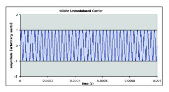
The black line running across the peaks of the wave is the envelope. Notice there is also a black line running across the troughs. This can also be used as the envelope boundary. As a rule, the lower envelope is a mirror image of the upper one. Below is the same 40kHz carrier, now being amplitude modulated by a 2kHz tone.
