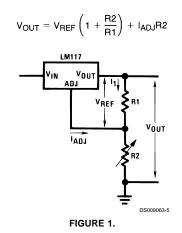
Since the 100  $\mu$ A current from the adjustment terminal represents an error term, the LM117 was designed to minimize I<sub>ADJ</sub> and make it very constant with line and load changes. To do this, all quiescent operating current is returned to the output establishing a minimum load current requirement. If there is insufficient load on the output, the output will rise.
