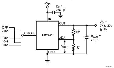
$$\begin{split} &V_{OUT} = \text{Reference voltage} \times \frac{\text{R1} + \text{R2}}{\text{R1}} \text{ where } V_{REF} = 1.275 \text{ typical} \\ &\text{Solving for R2: } \text{R2} = \text{R1} \left( \frac{V_O}{V_{REF}} - 1 \right) \end{split}$$
