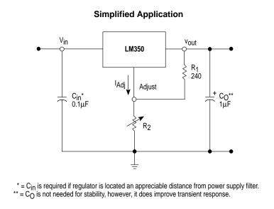
$$V_{\text{out}} = 1.25 \text{ V} \left(1 + \frac{\text{R}_2}{\text{R}_1}\right) + \text{I}_{\text{Adj}} \text{R}_2$$
