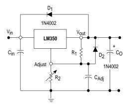
Figure 19. "Laboratory" Power Supply with Adjustable Current Limit and Output Voltage
