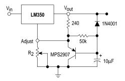
Figure 21. 5.0 V Electronic Shutdown Regulator
