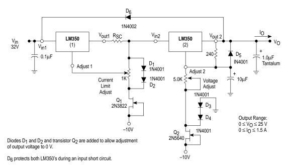
Figure 20. Adjustable Current Limiter
