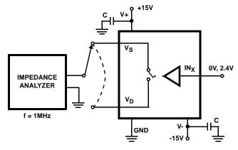
FIGURE 6. SOURCE/DRAIN CAPACITANCES TEST CIRCUIT
