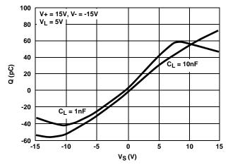
FIGURE 12. CHARGE INJECTION vs SOURCE VOLTAGE
