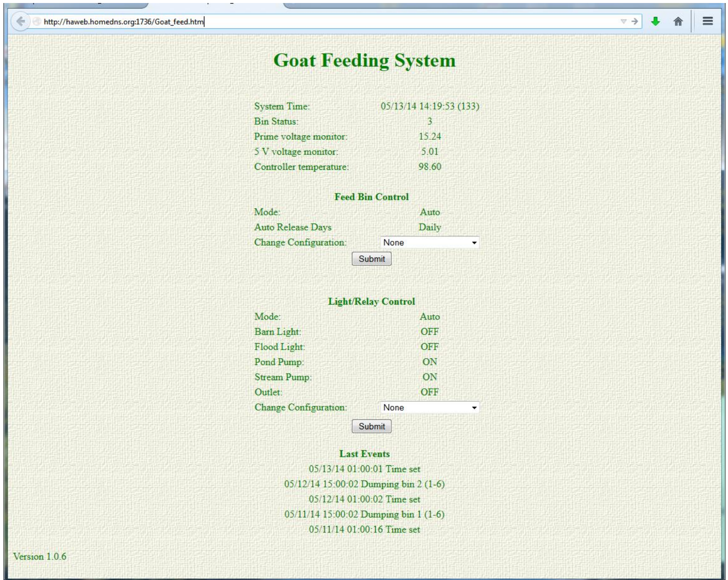
Figure 4 Control/Monitoring Web Page – This webpage is generated by the web server built into the control system. The web interface provides a quick way to monitor the operation of the system. It is also possible to manually control the system via this web page if desired.
