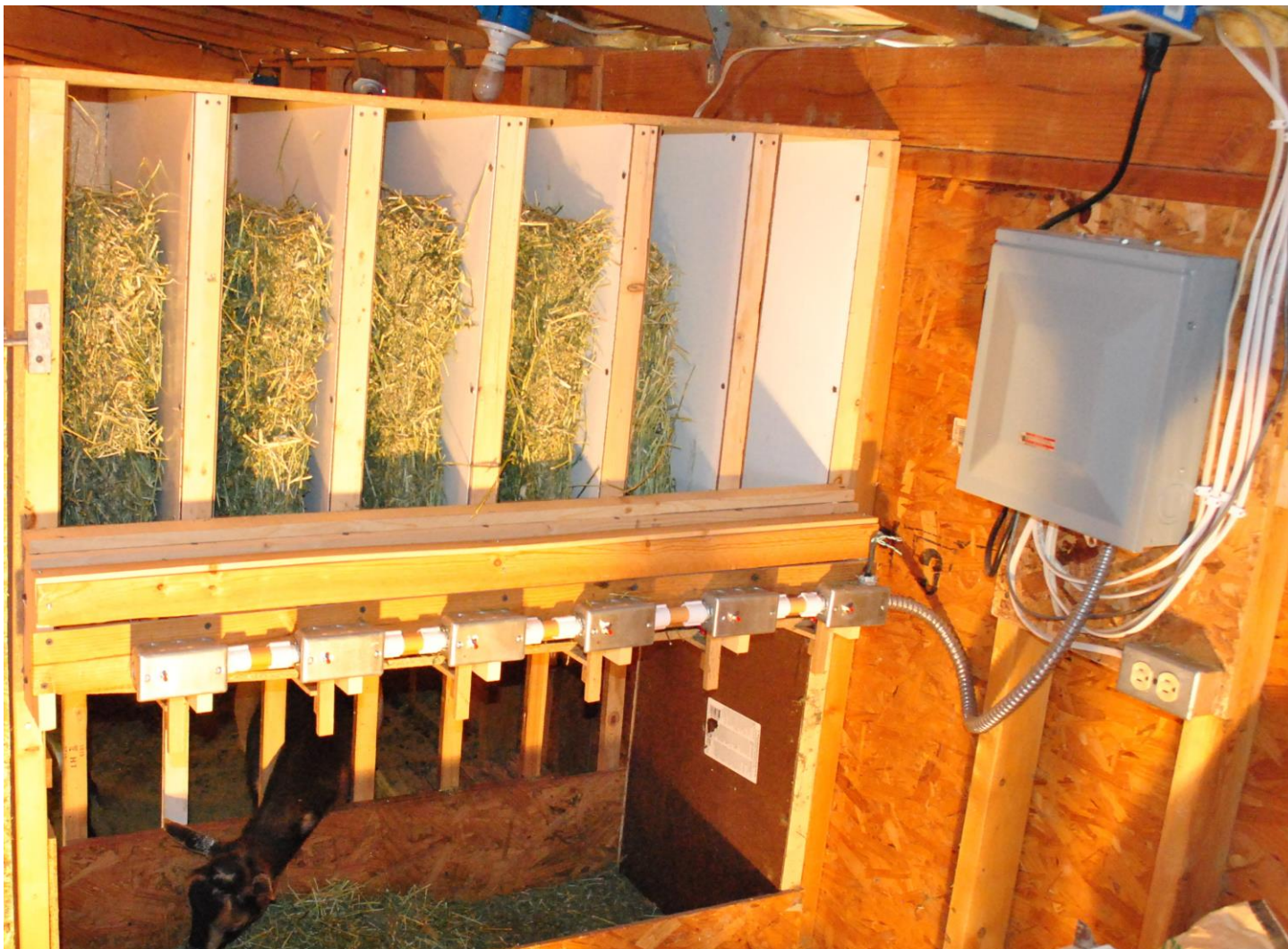
Figure 2 Photo of Completed Automatic Animal Feeder System – The six feed bins are shown in the upper left portion of the photo and the gray electrical box on the right contains all the control electronics to control the feeder. The electronics also contains a web server to provide remote control and monitoring via the Internet.
