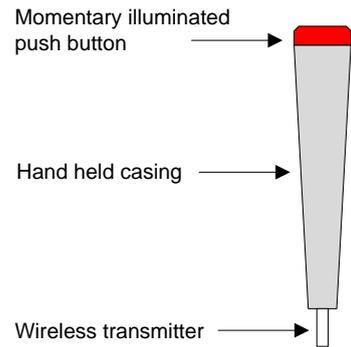
Maximum distance between transmitters and receiver 25m
