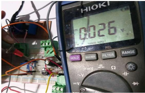
Q3 drain and Q3 gate voltage is 12.05 v
