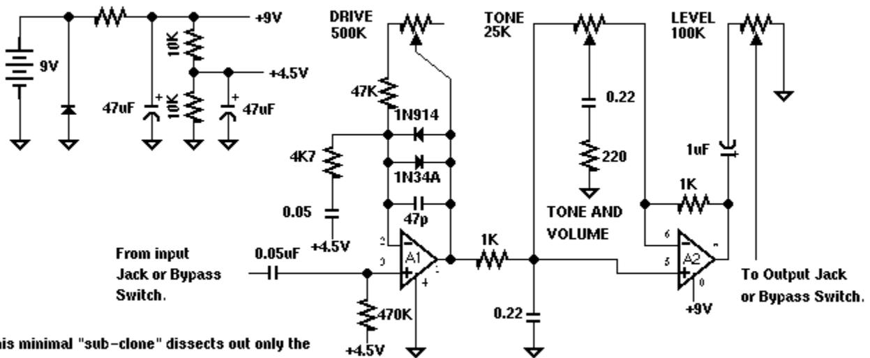
This minimal "sub-clone" dissects out only the clipping stage and tone/volume stage, leaving only the dual opamp and supporting parts. It relies on the high input impedance of the clipping opamp and the low output impedance of the Tone/volume opamp, and a true bypass switch arrangement.
