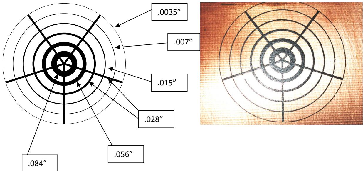
Successful test at measuring temp of back of board temp not face temp.( board must come completely up to temp.) at 255°F. Whatever time this takes is irrelevant only that whatever heat setting you use do not let the back of the board exceed 255°F. Any lower than this and the toner does not stick. Any higher than this and you are liquefying the toner. This is the best way to measure fusion temp. PC board used is  $\frac{1}{2}$  oz copper double sided, .064" board thickness.
