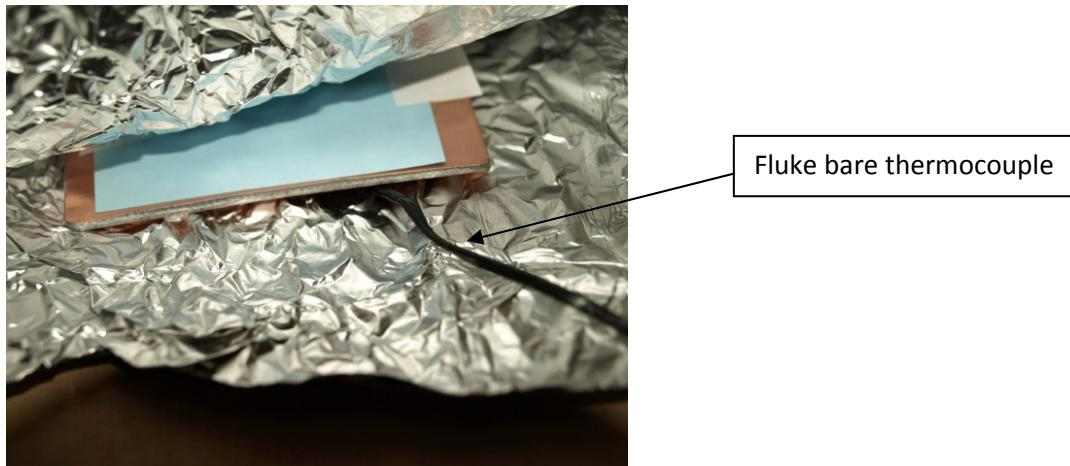
After board reaches temp, on the press bed (blanketed for insulation) and off of the foil (to aid in heat distribution) I immediately roll it out with a rubber laminate roller with 5 back and forth rolls reverse the
