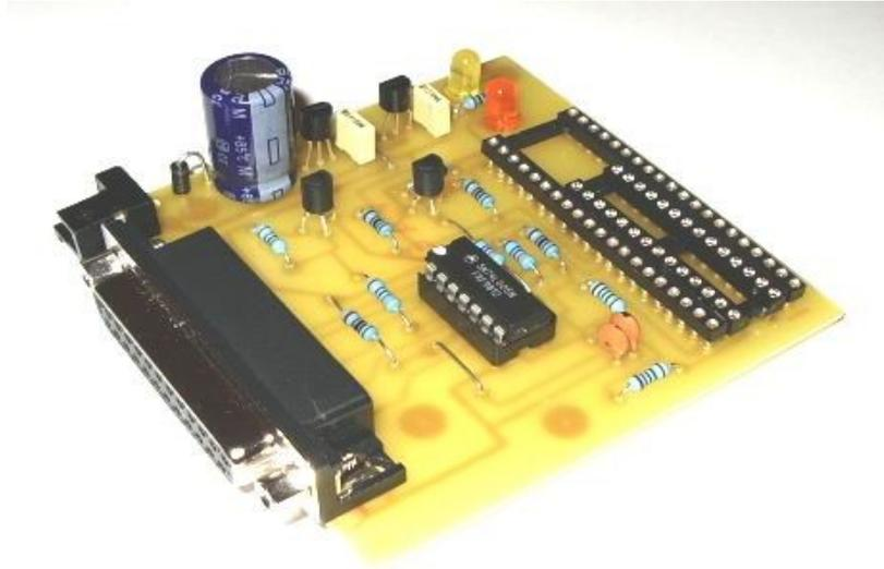
The 28pin/40pin Parallel Port PIC Programmer for the the project chips.
