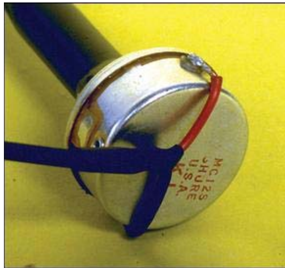
. . . and from the opposite side, with the connections to the shield cable which goes off to the preamp.
