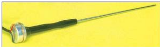
The completed "probe" which is actually a dynamic microphone insert Araldited to a long-bladed screwdriver.
