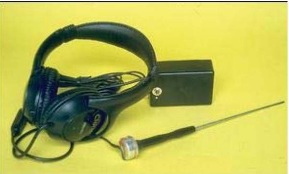
Here's the direct connection Snooper. Both it and the Parabolic mod use almost identical electronics - the main difference is th microphones and their mounting.
