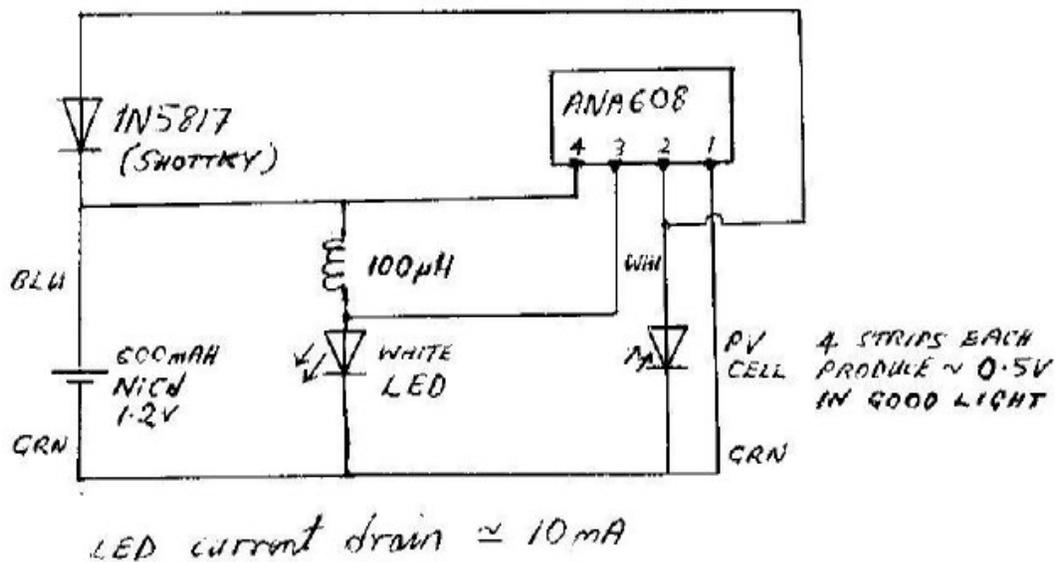
The ANA608 is the LED driver IC and works in a similar fashion to a DC-DC switched mode voltage up converter. There are only 5 other components, the Photo-Voltaic cell array, a white LED, a 100uH inductor (I mistakenly identified this as a resistor first – thanks to Gareth G4XAT for putting me right), a Schottky diode and a Ni-Cd cell. Below are pictures of the innards:
