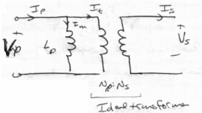
$$I_p = I_m + I_t = \frac{V_p}{j\omega L_p} + \frac{N_s}{N_p} I_s = \frac{V_p}{j\omega A_\ell N_p^2} + \frac{N_s}{N_p} I_s$$
