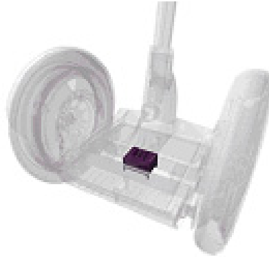
Figure 2.14: Diagram of location of balance sensors assembly on the Segway (Segway Inc 2005)
