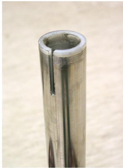
Figure 5.19: Photograph of nylon sleeve used in post clamp assembly
