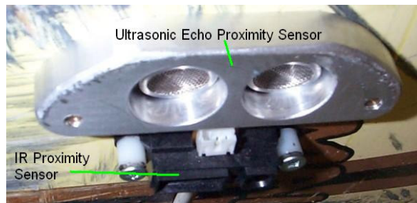
Figure 2.29: Photograph of proximity and Infra-Red sensors on Project Emanuel skateboard (Chudleigh et al. 2005)
