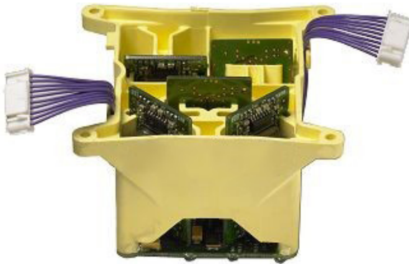
Figure 2.13: Photograph of Segway Balance Sensor Assembly (How Stuff Works Inc 2005)
