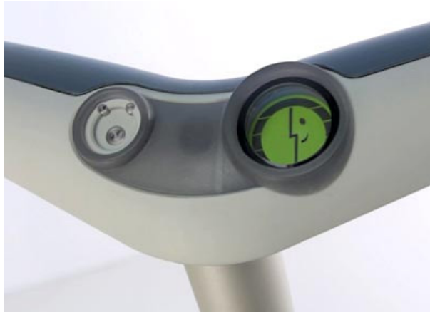
Figure 2.15: Photograph of Segway handlebar, showing key system and LCD (Segway Inc 2005)
