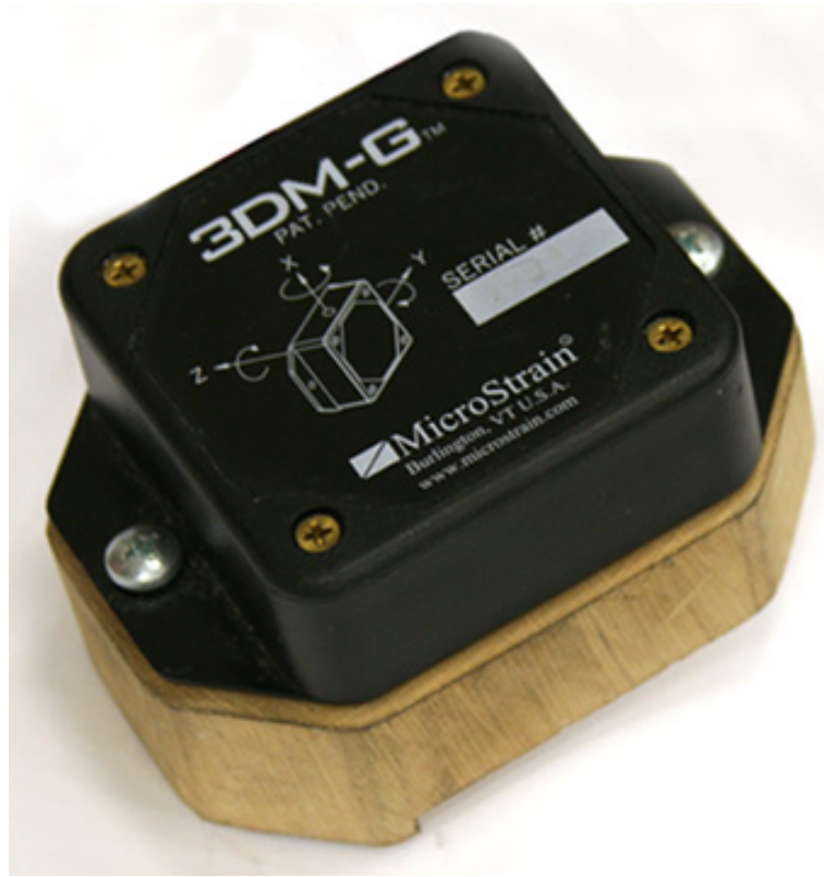
Figure 7.10: Photograph of the IMU mounting assembly
