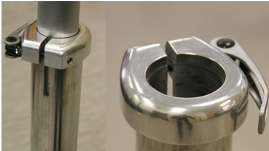
Figure 7.9: Photograph of the height adjustment mechanism
