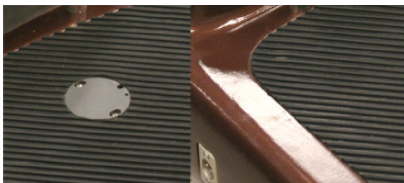
Figure 7.19: Photographs of the rubber mat showing a capacitive sensor
