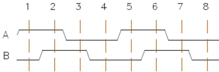
As shown, both channels A and B wrap around on themselves. When either signal changes, the state of one signal (say new B) is xor'ed with the previous state of the other signal (in this case old A). It does not matter which old signal is xor'ed with which new signal so long as the choice is always the same. The trigger for making a comparison is a change in state of either signal.
