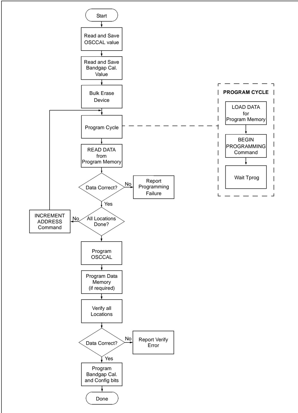
FIGURE 2-13: PROGRAM FLOW CHART - PIC12F629/675 CONFIGURATION MEMORY
