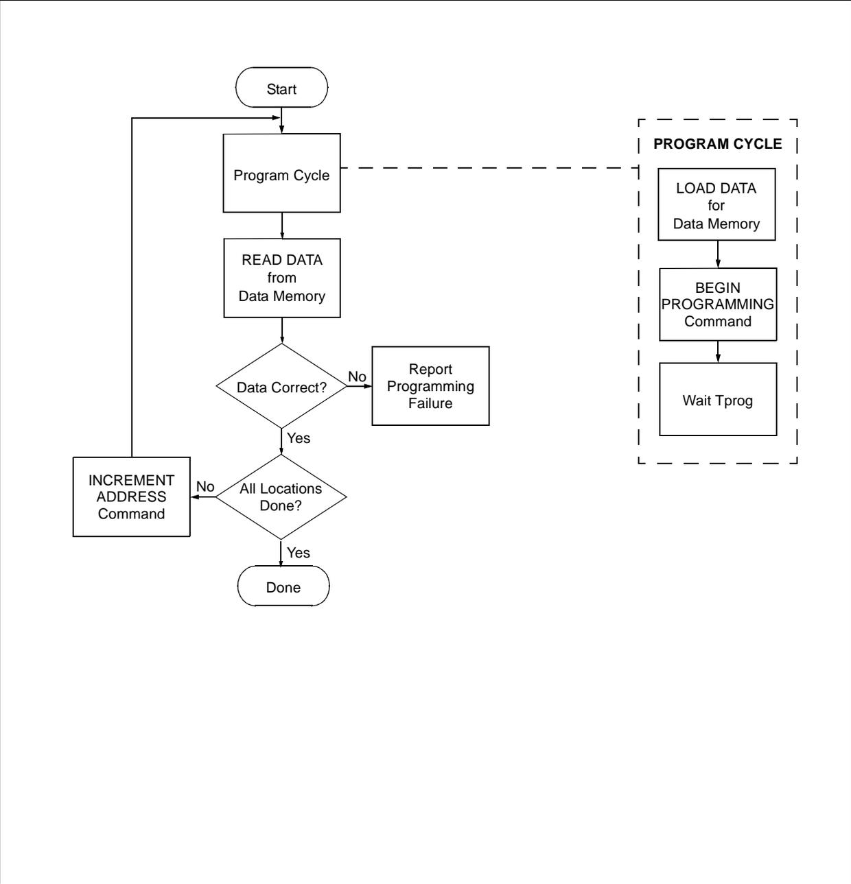
FIGURE 2-15: PROGRAM FLOW CHART - ERASE FLASH DEVICE
