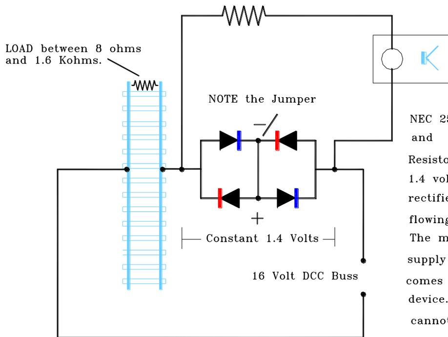
NEC 2506 Data states that op current is 10Ma. and Max AC voltage is 1.4 volts. The 33 Ohm Resistor drops the voltage to about 1.17 (Typical). 1.4 volts is developed across the 2 or 4 Amp bridge rectifier. This voltage is independent of the current flowing through it.
