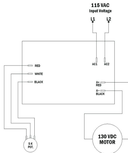
PWM control mod: Most of the information was posted by Jroque on: <http://www.cnczone.com/forums/showthread.php?t=8579>
