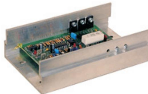
These SCR motor controllers are physically identical. The only difference is in the components used to allow a higher Current Limit on the MC-64 and a lower Current Limit on the MC-67. The MC-60M controller is a variation of the MC-60 controller that allows a single wire harness to carry signals between the console and controller. The treadmill's reed switch plugs into the controller, then the tach signal from the reed switch and the speed control signal are sent to the console.
